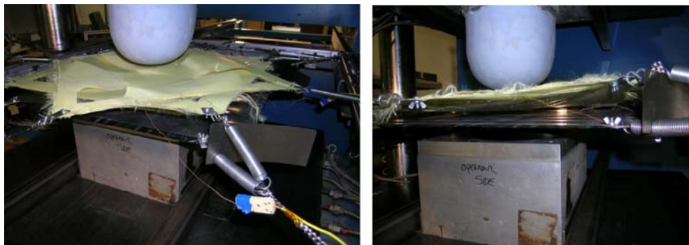
Figure 10. Blank fixturing and alignment of the plies within the press
